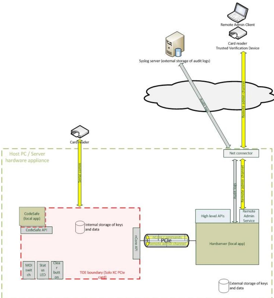
Figure 4 Configuration 2: TOE in host server
